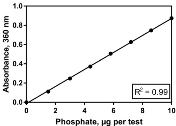
Figure 2. Linearity of the phosphate assay.
