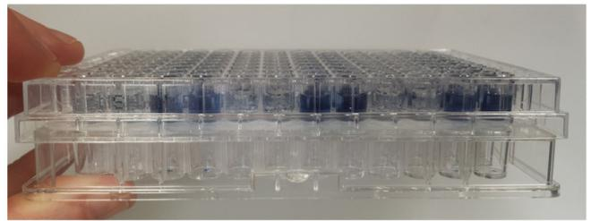
d. Sandwich the plates together as above, ensuring to align the plates in the same order to avoid confusion. Centrifuge at 2,000 x g for 10 min.
