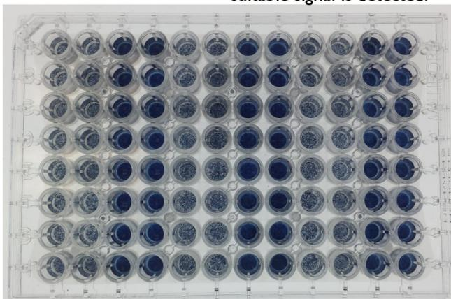
c. The reaction plate after incubation at assay temperature and for an appropriate time (e.g. 40°C for 10 min).
