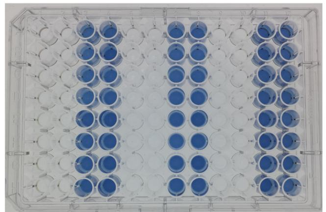
f. The catch plate after centrifugation. The plate is now ready to be read spectrophotometrically at the appropriate wavelength for the insoluble substrate (e.g. 590 nm for AZCL substrates as here).
