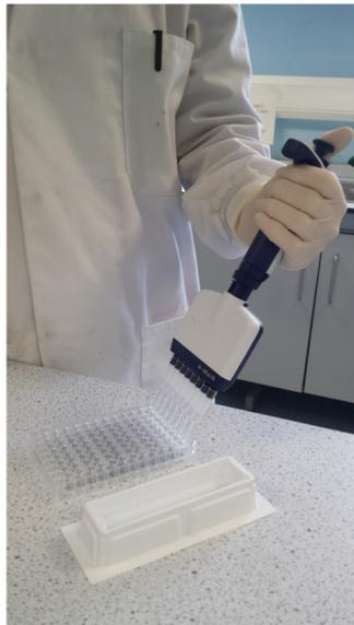
b. Pipette the enzyme solution into the reaction plate. Ensure that the plate and enzyme solution has been equilibrated to assay temperature. Include a reaction blank (assay buffer only). Incubate the plate at assay temperature until a suitable signal is detected.
