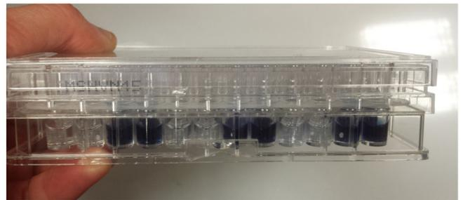
e. Reaction and catch plate after centrifugation. All the liquid should have transferred into the catch plate.
