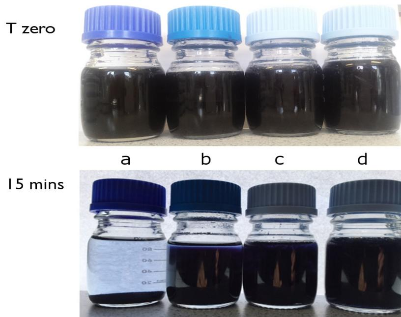
**Figure 3.** The effect of xanthan gum on the rate of settling of insoluble dyed substrate; time zero and after 15 min. Bottles a-d contain 0.2% w/v insoluble substrate with varying concentrations of xanthan gum. a) 0% w/v xanthan gum, b) 0.05% w/v xanthan gum, c) 0.1% w/v xanthan gum and d) 0.5% w/v xanthan gum.
