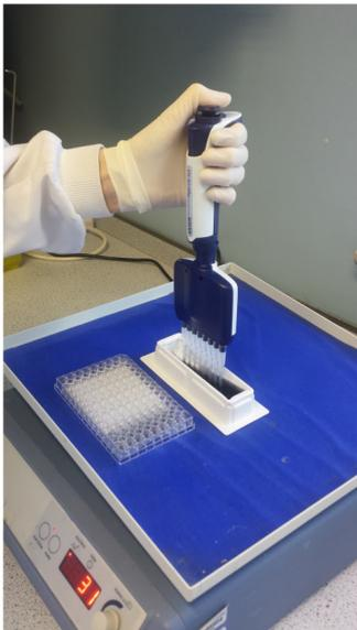
a. Pipette the insoluble substrate into the reaction plate ensuring that the solution is agitated at all times. This will prevent the settling of the insoluble substrate.
